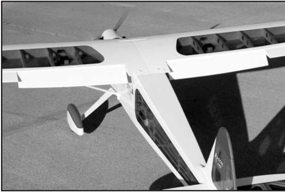
Flaps in full down position. It is common practice to mix in a small amount of down elevator as the flaps come down, to eliminate any tendency for the airplane to balloon up.
