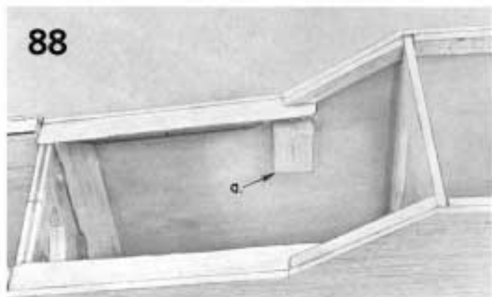
88. a. Place small blocks on each side of the fuselage to hold the tank centered. Don't get the blocks too tight, just enough to keep the tank from rattling around and yet release the tank easily for removal when needed.
