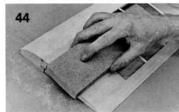
44. Sand the center section planking and cap strips even.
