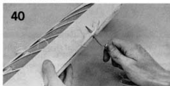
40. Carve the leading edge to airfoil contour.
