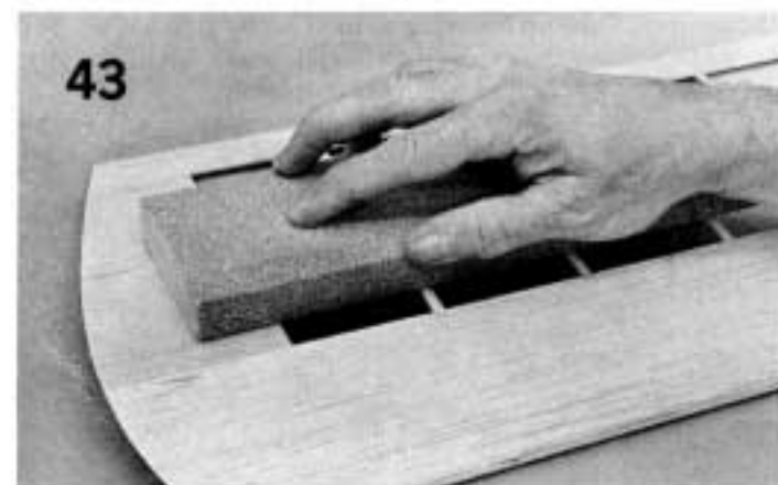
43. Sand the top of the cap strips and tip planking even.
