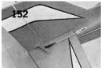
152. a. Cut out a slot for the pushrod exit.
