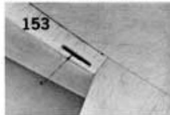
152. a. Cut out a slot for the pushrod exit.
