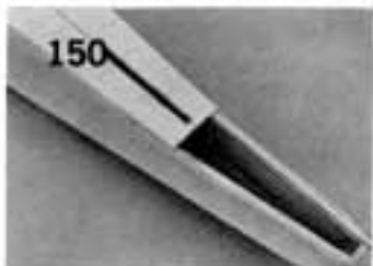
150. Cut out the slot.
