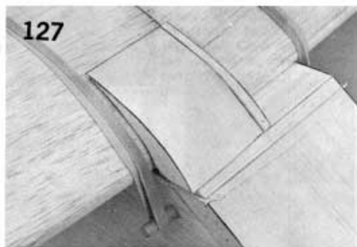
127. Fit the rough cut wing-cabin fairing blocks into place.
