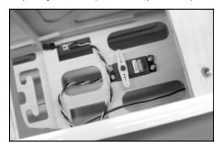
□ 6) The throttle servo is now installed. This servo is positioned into the fuselage servo tray, next to the throttle pushrod. To allow for full movement of the pushrod, position the servo with its output arm toward the rear of the fuselage, as shown. Install the grommets and eyelets onto the servo and use the screws provided with your radio system to secure it in place onto the tray.
