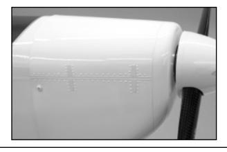
□ 12) With the engine temporarily back on the mounts, the required hole for the throttle tube is marked onto the face of the
