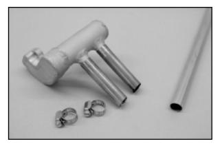
In order to allow the exhaust extensions to be clamped in place, it is necessary to first "slice" them at one end, in four places. These slices are made with a Dremel® Tool and a carbide cut-off wheel. Make each slice about 3/8" deep.
