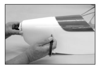
Use a 1/16" dia. bit to drill guide holes into the fuselage, about 1/4" deep. Use the four #3 x 10mm PWA screws to mount the cowl to the fuselage. Do not over-tighten these screws at this time. Remove the screws and the cowl, for now.
