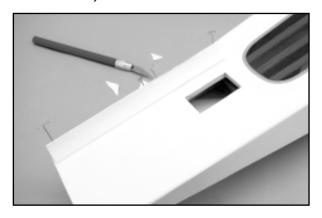
□ 3) Looking inside the elevator servo opening, you will see the factory installed pull-pull exit tubes. These two exits are now opened on each side of the fuselage, as shown. After finding
