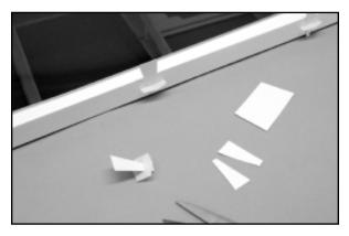
Flex the aileron downward, exposing the hinges between the wing and aileron. Hold the aileron in this flexed position with a piece of masking tape. For CA hinges, we always recommend using a
