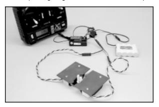
If you are using a computer radio, you can easily center the two servos through the radio's program for that function.
