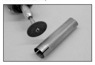
Remove any burrs that may be in the way and slide the tubes sliced ends first - onto the muffler's exhaust tubes. Position the tubes at the same length with each other and use the hose clamps to secure them firmly in place.
