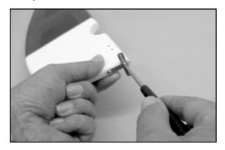
□ 7) The tailwheel assembly is now mounted to the fuselage. Note that the bottom rear of the fuselage has a plywood hardpoint beneath the covering for mounting this assembly.
