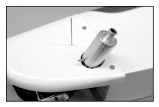
Cut a new length of 1/16" music wire, about 4" long. Put the cowl back on the fuselage and insert one end of the wire through the cowl and into the hole in the needle valve. Tighten the setscrew enough to hold the wire. Use a marker pen to mark the wire, outside of the cowl, about 1/8" away from its surface. Remove the wire from the needle valve and cowl. Use pliers to make a 90° bend at the mark just made. Trim the excess wire from the bent
