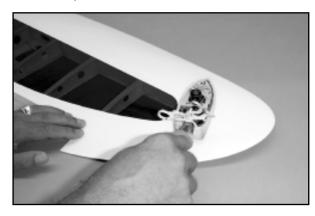
We also suggest that you take a few moments to go over all the seams with your iron, making sure they are all sealed and well adhered. This is especially important when you power your model with a glow engine. Exhaust residue will contaminate a seam that is not sealed, making it almost impossible to re-seal effectively.
