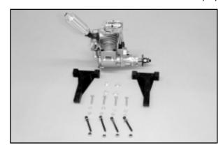
The first step is to properly mount the engine itself to the motor mount arms. A very easy and accurate way to do this is to temporarily mount the two motor mount arms onto a scrap piece of 1/4" plywood, with the correct spacing for your engine. Doing this ensures that the <u>back</u> faces of both mounts are truly flat in
