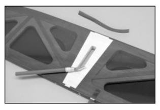
Use 5-minute epoxy to glue the stab in place to the fuselage. Apply glue evenly to the stab saddle at the top rear of the fuselage. Also, apply glue to the exposed wood on the bottom center of the stab. Place the stab onto the fuselage, making sure it is centered in top view as well as in front view. Use weights or pins to hold the stab in this aligned position until the epoxy cures. Clean off any excess glue on the bottom of the fuselage/stab joints with alcohol.
