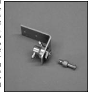
We mounted our fueling valve on the firewall, pointed straight down through the bottom cowl opening. Be sure to locate the bracket far enough off center on the firewall to allow your glow driver to fit onto the glowplug. Mounting the bracket in
