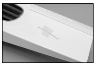
servo compartment, avoiding the stringers or the rudder cable extension. These cables must be unobstructed, with a straight run to the servo. Reach into the fuselage and pull the cable into the servo compartment. Use a piece of tape at the rear of the fuselage, to hold the cable end in place.
