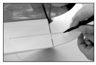
Place the control horn onto the line just made, centering its base on each side of the line. In top view, line up its four linkage holes with the hinge line of the rudder. Hold the horn in this position and use a marking pen to mark the two base mounting hole locations
