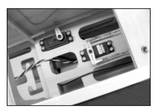
□ 8) The throttle pushrod is now connected to the throttle servo. Plug the throttle servo into the receiver and turn the radio system on. Use the transmitter to check the throttle servo for the correct direction of travel for "high" and "low" throttle - reverse the servo travel, if needed. Place an output arm onto the servo, positioning it to provide equal travel in both directions. Turn the radio system off, for a moment.
