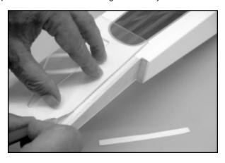
Use 5-minute epoxy to glue the two fairings in place onto each fuselage side, flush with the top surface of the stabilizer saddle, as shown. Pin the fairings in place and allow the glue to cure.
