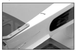
□ 3) **IMPORTANT:** We urge you to take a few minutes to cut and fit short lengths (about 3/16" or so) of medium fuel tubing onto all of the R/C links on the airplane. This simple safety precaution keeps these connections secure and safe.
