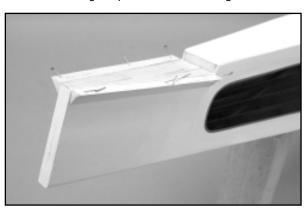
2) On the <u>right</u> fuselage side, directly beneath the stabilizer saddle, there is an opening for the elevator servo. The opening has been covered over at the factory and must now be opened. Use a hobby knife with a sharp #11 blade to do this now. Find each corner of the rectangular opening and cut the covering toward the center, leaving four covering "flaps". Use a small covering iron to seal the four sides of the opening and trim the excess material away.
