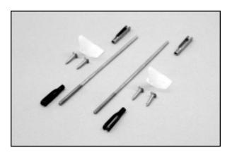
The two #4-40 solder links are now soldered to the unthreaded ends of each #4-40 x 4-3/8" pushrods. To make this easy, quick and strong, we highly recommend using Stay-Brite® Silver Solder and flux - available at most hobby shops. You will also need a good soldering iron (25W or better) or gun. Lightly sand the unthreaded end of both pushrods, where the solder link will be positioned. This tends to make the solder joint even more secure. The secret to
