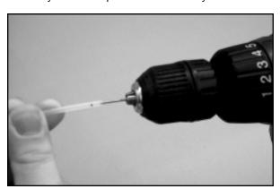
an electric drill. Lightly chuck the stud about halfway into the drill and holding the nylon pushrod firmly, thread the stud in place with the drill - simple, neat, and quick!
