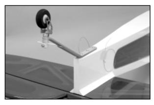
□ 8) The rudder is now hinged to the vertical fin. The method for doing this is exactly the same as it was for the ailerons and elevators, hinged earlier in this manual. After letting the CA glue wick fully through the hinges and surrounding wood (about 10 minutes), flex the rudder firmly in each direction to create free and easy movement.
