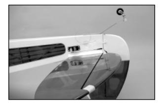
Adjust the R/C link in or out on the pushrod, until the base of the control horn sits exactly at the edge of the bevel line on the elevators. With the base of the horn in this position, mark the location of its two mounting holes onto the elevators, using a sharp pencil or pointed object. Turn the radio system off and remove the output arm from the servo, with the pushrod still in place. Remove
