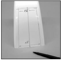
the measurements, connect the marks with a non-permanent pen and a flexible straight edge, such as a strip of balsa. At the top of the opening there are two corners. Use a circle guide to draw radiuses at these two corners.
