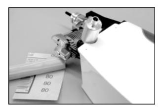
The open wood in the channel needs to be filled and fuel proofed. Use a little 5-minute epoxy to do this, smoothing it with your finger. When the glue sets, sand it smooth with 220 sandpaper.
