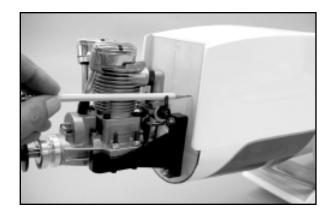
firewall. Visually line-up the throttle arm, at the point where it will be driven by the throttle pushrod, straight back to the firewall. Use a pencil to mark this location on the firewall.
