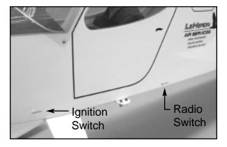
switch inside the fuselage, on the floor, just ahead of the landing gear block placing it far forward, away from the radio system. To activate the switch, we used a piece of music wire with an "L" bend, on the fuselage side. To do this like we did, refer to the Radio Installation section, Step #1.
