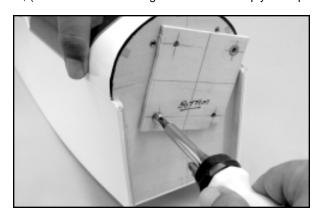
first in order to avoid "dimpling" the face of the firewall with the bolt head).
