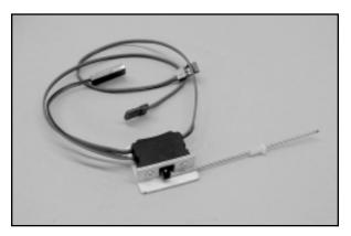
□ 2) The receiver is now placed in the fuselage. Connect the servo leads to the appropriate channels in the receiver, including the aileron "Y" harness and the switch connector. Test the radio system first, making sure everything works. The receiver is wrapped in protective foam, held in place with tape or rubber bands. The two aileron cable ends of the "Y" harness should be both free and accessible from the top of the cabin. We placed our
