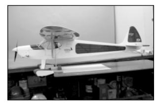
The goal is to get the airplane to balance perfectly level at the desired C.G. point. Level means level - not nose down or tail down - level! If the nose hangs down, the model is nose heavy. Likewise, if the airplane hangs tail down, it is tail heavy. If either of these conditions exist with your model, they must be corrected.
