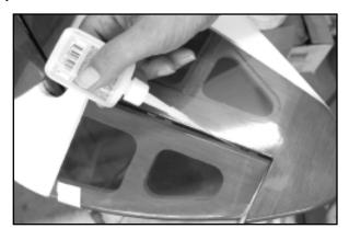
The two nylon rudder control horns are now mounted in place, one on each side of the rudder. In case the bottom rudder hinge interferes with the two horn mounting holes, use a 5/64" drill bit to clear the holes. From the kit contents, locate two nylon control horns, two M2 x 20mm Phillips head bolts and two M2 hex nuts.
