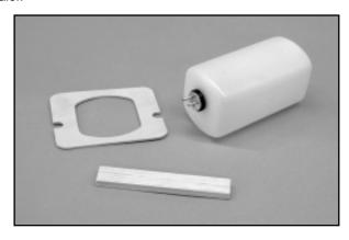
Cut two 8" or so lengths of fuel tubing and place one length onto each of the two fuel tank lines. Fish a length of string through the round fuel tank hole in the firewall, through the tank compartment and into the cabin area. The string will be used to direct the tank and fuel tubing into the tank compartment. Tie the end of the
