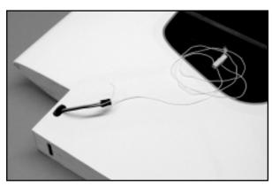
Both aileron servo hatches are now secured in place into each wing panel, using the eight #3 x 10mm PWA head screws.
