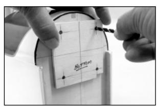
□ 3) The scrap piece of plywood used to mount the engine has now become a pattern that is used to accurately locate the four
