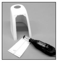
Follow this by using a drum-sanding bit to smooth the edges and contour the corner radiuses. Be careful to keep the edges as smooth and uniform as possible, using the lines as a guide. Use a sanding block with 220-grit paper to sand the straight edges smooth. Finally, use a piece of 220 sandpaper to lightly sand all of the edges, making them completely smooth. Clean the cowl, removing all dust and wipe off any remaining ink lines with alcohol.
