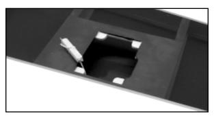
Also, on the bottom of each wing panel, at the center front location, you will see an oblong opening. This is the aileron servo lead exit opening. Inside this opening, you will see a piece of wood with a
