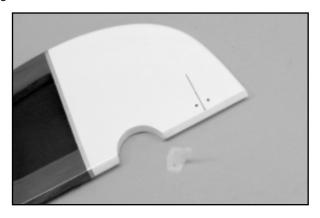
□ 6) The two-arm rudder steering plate is now attached to the bottom leading edge of the rudder, as shown, using two #2 x 10mm PWA screws. Note that the bottom leading edge of the rudder has hardwood beneath the covering as a mounting base for these screws. Position the front edge of the horn 1/8" behind the leading edge of the rudder and use the horn's mounting holes as a pattern. Drill two 1/16" dia. guide holes for the screws. Secure the horn in place with the screws.
