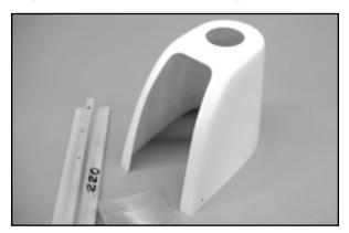
The cowl should now be able to fit over the engine and onto the front of the fuselage.
