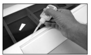
fine-tip applicator on the glue bottle, to better control the flow. Remove the card wedge from one of the hinges and carefully apply four (4) small drops of thin CA glue to the left and right side of the exposed hinge center.
