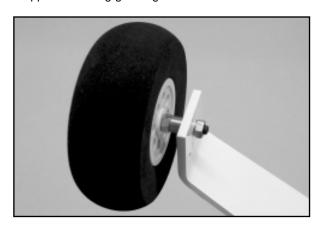
b) Note that there is a <u>front</u> and <u>rear</u> edge to the aluminum landing gear. In side view, the leading edge (or front) of the landing gear is straight. The trailing edge (or rear) is slightly angled. Be sure to mount the landing gear and the self-aligning wheel pants in the correct direction!
