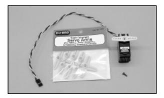
the front. You will need an output arm that is long enough on each side to properly operate the pull-pull linkage to the rudder. As mentioned earlier, we used the Du-Bro "Super Strength Servo Arms" for all of our servo output arms. We used the 1-3/4" two-arm output for the pull-pull set-up on our rudder servo.
