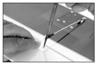
Once in position, use a pointed object to mark the control horn's two mounting hole locations into the aileron. Rotate the pushrod out of the way and use a 1/16" dia. bit to drill two holes - about 1/2" deep - into the aileron at the marks just made. Remove the control horn from the R/C link and use two #3 x 12mm PWA screws to mount the control horn securely to the aileron.
