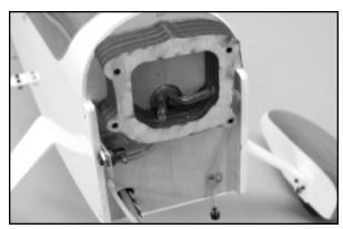
□ 4) If your engine has a Pitt's style muffler, it will probably require exhaust extensions to clear the firewall at the bottom of the fuselage. In the case of our F.P.E. 1.3, we used two 2-1/2" lengths of K&S brass tubing, 17/32" in diameter (K&S #140). This tubing had the perfect inside diameter to slip over the F.P.E. Pitts muffler.
