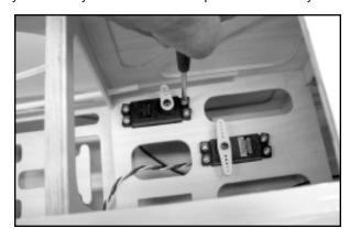
□ 7) In this step, the pull-pull cables are attached to the rudder servo output arm. The connection of these cables to the rudder will take place in the Tail Group Assembly section. Uncoil one of the pull-pull cables. Thread one end into one of the pull-pull exits at the rear of the fuselage side. Carefully feed the cable toward the
