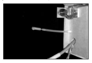
Insert the opposite end of the nylon pushrod into the female tube at the firewall and push it in place all the way back to the servo bay. Press the nylon ball link fitting onto the ball link on the carburetor throttle arm. The servo end of the pushrod will be prepared after the throttle servo is installed in the coming steps.
