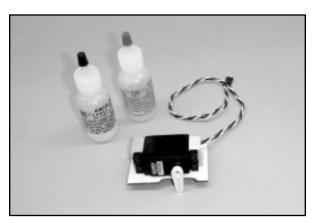
First, position the servo with its output arm directly over the center of the hatch's clearance slot and centered in the middle of the "1/2 slot" cut-out. Allow the glue to set. With the servo mounting blocks now glued in place, remove the servo. Assemble the remaining servo hatch cover and servo mounting blocks in the same manner.
