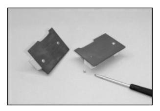
Use the servo mounting screws provided with your radio system to secure both aileron servos in place to the mounting blocks on each aileron servo hatch. To avoid possibly splitting the mounting blocks with the screws, first pre-drill the holes with an under-size drill bit.
