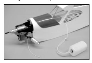
string at the cabin area firmly to the ends of the two fuel lines.
