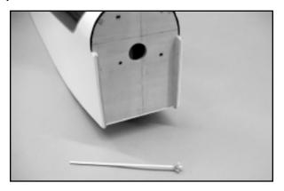
Hold the nut against the firewall with your finger and use one of the M4 bolts to engage its threads from the front of the firewall. Thread the bolt all the way in place. Use a screwdriver to tighten the bolt, "pulling" the barrel of the blind nut fully into the back side of the firewall, (we ran our bolts through the holes in the plywood pattern
