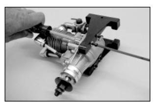
Apply a little threadlock compound to each of the M4 x 25mm mounting bolts. Slip a split ring washer and a M4 washer onto each bolt. Hold the engine/motor mount assembly in place to the firewall and install each bolt in place to hold the assembly to the firewall. Allow enough play in the bolts to be able to slide the motor mount arms left or right, as needed, to center the motor mount bases to the firewall. When everything looks about right, firmly tighten the bolts.
