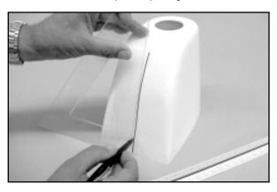
Since the overall width of the Saito 1.50, at the head, is about 2-1/4", we know that the opening must be at least that wide. When creating this opening, the idea is to neatly expose as much cooling air to the cylinder head as possible. As shown, we used a width of 3-1/2" at the back of the cowl, tapering up to 2-1/2" wide at the top of the opening. After making
