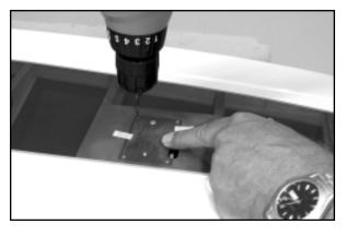
Re-drill the four corner holes in the servo hatch, using a 1/8" dia. bit to allow clearance for the #3 screws. The aileron hatch covers are now complete and ready for mounting.
