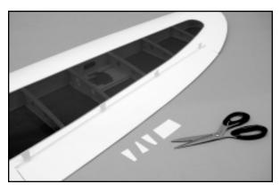
Press the four hinges into the slots in the wing panel, up to the hinge's center slot. Place one of the card wedges into each hinge, then press the aileron in place onto each exposed hinge half, up to the card wedges. Slide the aileron left or right to center it within the wing panel aileron bay. The hinges are now in proper position for permanent mounting.
