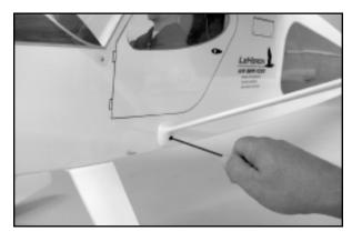
An easy way to store and transport your wing struts is to use thin foam to wrap each end of both struts. This separates them and protects the end fittings from damage. Between flying sessions, leave the strut bolts installed in the wing panels and fuselage sides to keep them from becoming lost.
