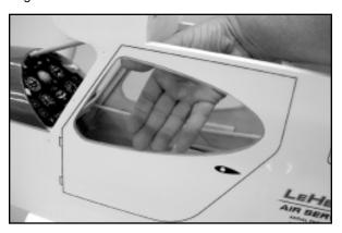
The windshield - removed earlier - is now re-installed back onto the fuselage, using the seven mounting screws. Likewise, the pilot figure is now re-installed into the fuselage.
