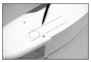
Use a Dremel® Tool with a drum-sanding bit to clear out the cowl, within the marks just made. Continue to trial fit the cowl in place to the fuselage, refining the cowl opening until it fits in place with a uniform 1/8" of clearance all the way around the muffler. With the openings made, use a wrench to tighten the manifold nut, securing the manifold in final position to the engine head. Likewise, tighten the muffler nut, locking it in place to the manifold.
