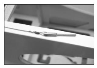
Thread the round, knurled locking "nut" all the way onto the threaded end of the pull-pull fitting and thread the R/C link in place. Leave equal an amount of threads exposed to make final adjustments later, when the opposite ends of the cable are rigged for the rudder horns.
