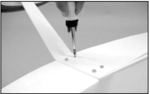
c) The completed landing gear assembly is now mounted to the fuselage using four M4  $\times$  20mm PWA mounting bolts and the four M4 split ring lock washers. Tighten these four mounting bolts firmly in place.
