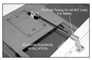
12) Repeat Steps 9, 10, and 11 for the second aileron. SAFETY ISSUE: After centering the servos and setting the control throws, "safety" each R/C clevis by slipping a short length of fuel tubing (not supplied) over the clevis, as shown in many of the photos. This will prevent the clevis from opening up and becoming disconnected from either the control horns
