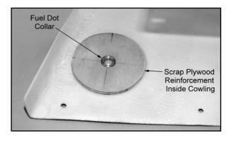
NOTE: If you do not want to put the fuel dot in the cowling, you can make a simple mount from 1/8" plywood that is glued and/or screwed onto the front of the firewall. Then make an opening in the cowling directly over the fuel dot, for access.
