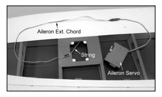
b. Repeat the previous step to tie the end of the flap retrievel string to the flap servo plug.
