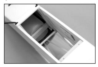
□ 9) Locate the pre-covered Tank/Battery Hatch from the kit contents. This hatch has a plywood "lip" at one end and two pre-drilled holes at the other end. The end with the lip is the front. The hatch fits into the bottom of the fuselage and is removable for ready access to the fuel tank and the battery compartment beneath the tank. Install the front hatch lip into the fuselage, beneath the landing gear spreader, pressing it firmly in place to the fuselage.
