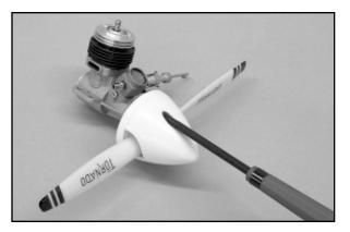
☐ 2) Place the engine onto the fuselage engine mount plate. The correct distance from the back face of the spinner to the very front of the fuselage is 1/4". Use a scrap piece of 1/4" balsa as a spacer on the left fuselage side and adjust the position of the
