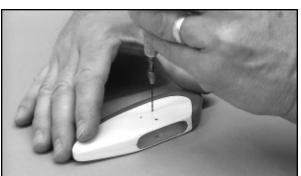
making these marks, remove the wheel pants from their axles. Use a pin vise and a .046" dia. drill bit (#56 numbered drill) to drill guide holes through the wheel pants and the inside plywood mounting pads, at the marks just made.
