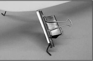
Use light sandpaper (#400 or similar grit) to lightly sand the trailing edges smooth and sharp. These fairings can now be finished with Oracover® film or primed and painted. Remount the wheel pants.
