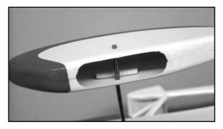
□ 2) The wheel pants must first be correctly aligned to the landing gear wire and the fuselage, before mounting. This is done by slipping the wheel pants in place over the landing gear wires - without installing the wheels - and then propping the rear of the fuselage up 3" off of a flat surface. This provides the correct side view alignment for mounting the wheel pants.
