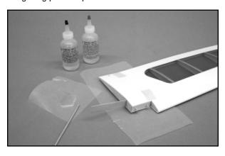
□ 3) After the glue has set, use the four provided 1/4" x 10" self-adhesive strips of white Oracover® film to cover the bottom and top wing joints, centering the covering over each joint. Save the
