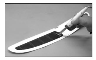
the wood to dimensionally "shrink" in the process. In turn, this may cause some relaxing of the covering. However, this is easily taken care of using a small heat iron, such as a small "trim seal" type unit.
