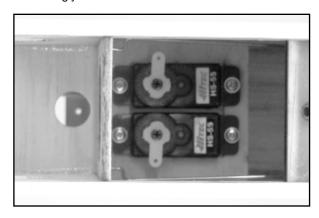
Remove the servo arms. Attach the wire elevator and rudder pushrods to the ends of each output arm. Place the arms back onto the servo output shafts and re-install the output arm screws do not tighten these yet because they may have to be repositioned when the radio system is tested and centered.
