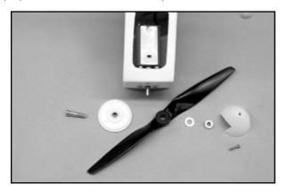
☐ 2) Press the aluminum collet firmly onto the motor output shaft at the front of the fuselage until it bottoms out. Slide the spinner backplate onto the threaded end of the collet, as far back as it will go. Slide the propeller onto the collet, back to the backplate. Install the washer onto the collet and thread the nut onto the collet threads. Align the propeller between the recesses in the spinner
