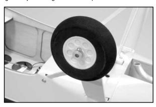
Now, fit the appropriate fiberglass wheel pant (there is a <u>left</u> and <u>right</u> pant) in place over the wheel, sliding its inner slot over the inner wheel collar. Determine if the fit of the wheel within the wheel pant is OK. Adjust the inner wheel collar on the axle as needed to position the wheel in the pant to roll freely. Tighten the setscrew to hold it in place. Repeat this fitting process with the opposite wheel and wheel pant.
