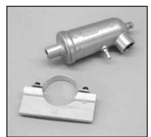
e) Last, we wanted to cushion the muffler when it is clamped in place into the muffler mount. To do this we slit a piece of heat resistant neoprene tubing lengthwise and placed it over the half-circle cut out, holding it in place with silicon glue. This custom muffler mount is now complete and ready to install into the fuselage. This will take place shortly so the mount handy.
