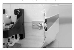
Lay a piece of 1/16" wide trim tape over the exact center of the valve, in a straight line back along the fuselage to a distance of about 8" or so. This tape will assist in locating the required opening in the cowl for the fueling valve.
