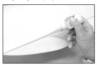
After sufficient time has passed, flex the hinged aileron firmly up and down on the panel to create free and easy movement. We also suggest pulling on each aileron, at each hinge location, making sure they are each firmly in place. Repeat this same procedure with the opposite wing panel and aileron.
