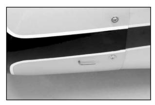
The only other thing that we would suggest is removing the extension from the needle valve and filing or grinding a small "flat" in its surface where the needle valve setscrew contacts it. This allows the setscrew to hold the extension firmly in place without loosening. Remove the cowl from the fuselage and set aside the needle valve and extension for later final assembly.
