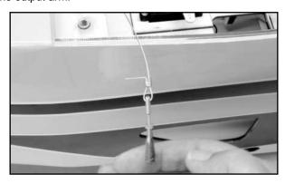
Install the clevis ends of the two rigging couplers onto the correct sides of the output arm, one in each outermost end and install and tighten the output arm screw into the rudder servo. Turn off the receiver and transmitter for now.
