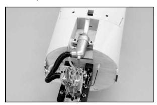
☐ 11) Reconnect the throttle clevis onto the carburetor throttle arm. Make all required fuel tubing connections to the fuel valve and the carburetor. The "vent" line goes back to the pressure nipple in the muffler. When fueling the tank, this line is disconnected for overflow purposes and then reconnected to provide manifold pressure to the tank.
