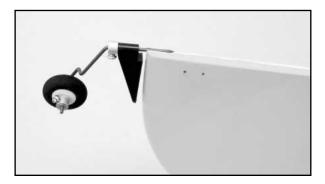
channel a little more to fully accept the tailwheel wire, making it flush with the hinge line. This can be done with a small file or a hobby knife with a #11 blade.
