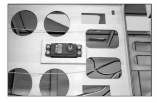
b) The rudder servo must now be neutralized, with the transmitter rudder trim also in neutral. Plug the rudder servo lead into the correct rudder channel in the receiver, followed by the switch and airborne battery pack. Turn on the transmitter and then the receiver. First determine that the servo is moving in the correct direction. If it isn't, use the servo reversing function in your
