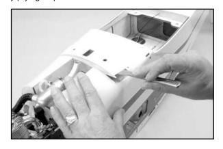
□ 2) Attach the nylon Center Landing Gear Wire Mounting Block in place onto the bottom center of the main landing gear, using two T2.6 x 10 mm PWA screws. This block is correctly in place with its slotted end facing downward in relationship to the landing gear. This slot accepts the main axle wire form when it's mounted in place.
