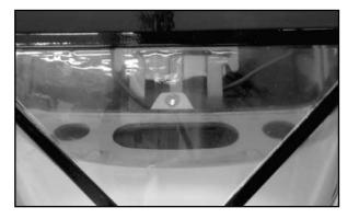
As shown, this installation requires a small hole to be drilled through the firewall to provide an opening for the glow plug connector wire and the ground wire. We secured our ground wire connector to the closest rear engine mounting bolt, using a metal connector crimped and soldered to the end of the wire.
