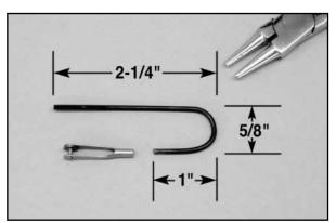
b) Using the M2 solder link clevis, solder the clevis in place to the short, unthreaded end of the pushrod. Note that the clevis is soldered to the wire with its two arms up on edge.
