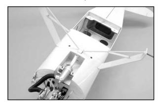
The axle wire form is now secured into the nylon block using the nylon "cap" and the two remaining T2.6 x 10 mm PWA screws.
