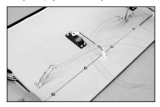
☐ 4) The remaining eight (either all left or all right-hand thread) turnbuckles are now installed onto the top surface of the bottom wing. As before, first adjust each turnbuckle for equal in and out adjustment. As shown, these turnbuckles are installed with their angled ends facing each other. Firmly tighten each mounting screw.
