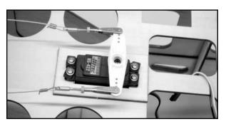
□ 14) The final pull-pull rudder connections are now made at the two rudder control horns. Use a piece of masking tape at the leading edge of the fin and rudder to hold the rudder in neutral to the fin. Turn the radio system on and turn the fuselage over, upside down on your work surface.
