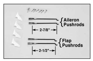
Pushrods (2-1/2" long with a metal clevis at one end and a Z-bend at the other). Locate Bag #21 and remove four (4) Nylon Control Horns and the eight (8) T2.6 x 12 mm PWA screws.
