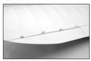
Flex the aileron downward, exposing both sides of the hinges, between the wing panel and the aileron. Use a piece of masking tape to hold the aileron in this position. Remove the card "wedge" from one of the hinges and apply four (4) small drops of glue to each side of the hinge slot. Remove the card "wedge" from the next hinge and again apply four (4) small drops of glue to each side of the hinge slot. Repeat this process with the remaining hinges.
