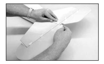
Center the elevators left and right to the stabilizer, leaving the same amount of clearance space at the outer counter balances.
