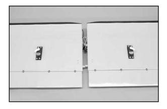
motion moves the output arms towards the flap, reverse the flap channel through the transmitter. With the servos now moving in the correct directions and the output arms in place correctly, linkages between the servos and the flaps can be safely made.
