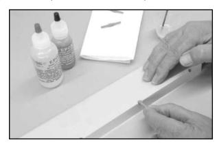
Each exposed hinge leg should be oriented  $90^\circ$  to the flap. Use alcohol and a paper towel to carefully remove any excess or oozing glue from the center hinge point and let the glue cure. Repeat this process with the opposite wing panel and its flap.
