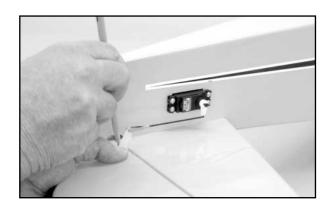
Rotate the control horn and pushrod out of the way. Use a #47 (.078" dia.) bit to drill two clearance holes for the M2 horn mounting bolts, completely through the elevator at the marks just made. Rotate the control horn and pushrod back into position and install the control horn to the elevator using the two M2 x 15 mm
