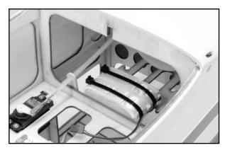
**On/Off Switch:** As mentioned earlier in this manual, we substituted the on/off switch that came with radio system for a MAXX Products #3470 *Charge Switch*. This heavy-duty aftermarket switch allows the airborne system to be charged externally and includes a silicon shock mount to prevent vibration damage. It is installed just like any other on/off switch.
