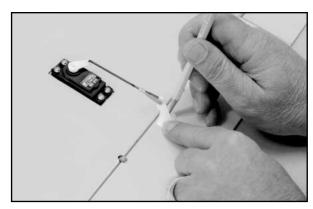
Using a #57 (.043") dia. bit, drill two parallel and perpendicular holes into the flap at the marks just made, about 3/8" deep. Repeat this on the remaining flap. Because the control horn mounting holes are undersize for the T2.6 mounting screws, use a #39 (.099") bit to open up these two mounting holes in each control horn base. The two flap control horns are now mounted to the flap using the provided T2.6 x 12 mm screws. Remove the tape from the top sides of both panels to free the flaps.
