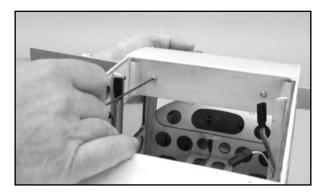
$\Box$  4) The molded windshield - removed earlier in these instructions - is now reinstalled in place at the top front of the fuselage with the four T2.6 x 8 mm PWA screws.
