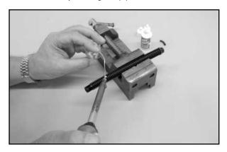
b) Disconnect the throttle linkage and remove the engine from the mount arms. Install one of the header nuts that came with the engine exhaust system and thread it fully in place onto the flex tube header. Thread the header in place into the engine exhaust port and firmly tighten the jam nut, locking the flex pipe in place in the engine.
