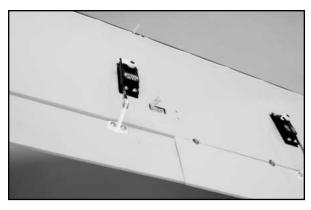
$\square$  12) As described in Step 2 of the Bottom Wing instructions, use one of the T2.6 x 8 mm PWA screws from Bag #22 to pre-thread the eight (8) rigging bracket holes. Return the screw to its bag for later use.
