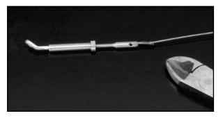
Repeat this process with the remaining seven turnbuckles, cables, and swages. You should now have eight turnbuckles with the flying wires attached and locked in place.
