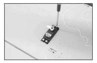
☐ 6) The flap servos are now installed in each wing panel. Like the aileron servos, the flap servos are oriented in the wing panel with their output arms facing outward toward the wing tip with the head of the servo toward the leading edge. Install the rubber grommets and eyelets into the mounting lugs of both servos.
