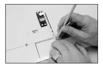
As you did when mounting the flap horns, use a #57 (.043") dia. bit to now drill two parallel and perpendicular into the aileron at the marks just made, about 3/8" deep. Repeat this on the opposite aileron. Use the four remaining T-2.6 x 12 mm screws to mount the control horns in place to each aileron. Remove the tape holding the flaps and ailerons together.
