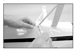
At the main landing gear legs, the forward ends of rear support struts intersect the small hole pre-drilled in each landing gear leg. Note that these support struts are mounted to the *inside* of the landing gear legs. Use the provided 4-40 round head Allen bolts and 4-40 lock nut to firmly secure the front of each support in place to the main landing gear legs. Now, go back to the previously installed bolts at the fuselage and tighten them.
