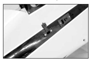
We mounted our well taped and foam padded sub-C cell on the bottom left side of the cabin servo tray, next to the receiver mounting location. A single zip-tie securely holds this cell firmly in place.
