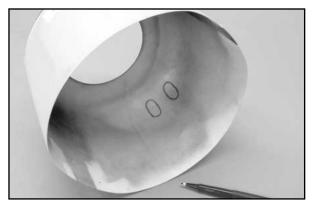
Now that these marks are clearly visible inside the cowl, they need to be transferred to the outside surface of the cowl. To do this we used a small flashlight held inside of the cowl to easily see the marks on the outside surface through the yellow paint. We again used a marker pen to trace these lines onto the outside surface of the cowl. If you don't have a small enough flashlight, use a bare light bulb - it works great.
