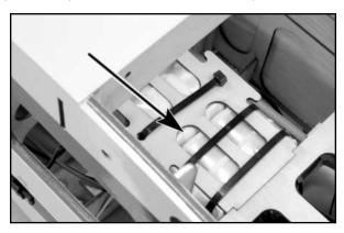
Last, the LED bulb needs to be mounted in a location that is easy to see. As mentioned earlier, we mounted our LED bulb against the forward fuselage cabin former, at the top. This location works well for us even on very sunny days. A scrap piece 1/8" lite-ply works great for this purpose. Simply drill it to accept the bulb and install it with against the former. Press the bulb in place and secure it with a drop of thin CA glue.
