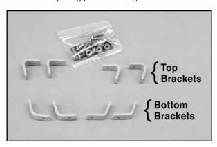
From the remaining small bag, select four of the  $4-40 \times 13$  mm bracket mounting bolts. Use a 2 mm Allen head hex wrench to now install the four N-strut brackets in place into the recesses in the top of the wing. We suggest using thread locking compound on the bolt threads and tightening the bolts firmly.
