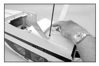
Now that the main landing gear is installed with the slotted nylon wire-mounting block in place, the fuselage landing gear hatch is now reinstalled in place into the fuselage, over the landing gear and nylon block. Center the hatch and use the two T2.6 x 12 mm PWA screws to secure it in place.
