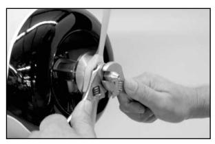
b) The spinner cone is installed over the propeller and into the backplate recess. Center the cone in relationship to the propeller blades, making sure the prop blade cut-outs are not contacting the propeller. The 8-32 x 9/16" socket head bolt is then installed into the center of the spinner cone and tightened in place.
