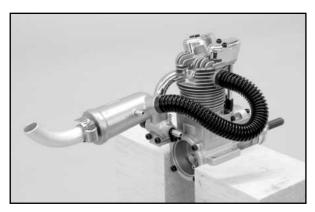
The engine, with the header, muffler, and diverter parts in place, is now final-mounted in place to the motor mounts using the recommended socket head bolts, washers and lock nuts. Tighten all bolts and nuts firmly.
