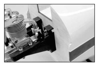
e) From inside the fuselage, slip both of the laser-cut plywood Throttle Tube Mounts onto the throttle tube housing. These mounts are used to direct and secure the throttle tube back to the throttle servo. They are glued in place to the cabin former and servo tray to create a smooth transitional curve back to the throttle servo arm location. Use 5-minute epoxy or thick CA glue to secure these tube in the mounts.
