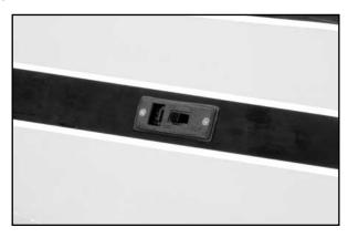
**Optional Glow Driver System:** The optional glow driver system is installed now. After completing the wiring of this system, the first thing to do is to mount the external charging receptacle that is provided with the product. Like the airborne on/off switch, we mounted this receptacle centered within the black trim stripe on the left fuselage side, as shown. Note the small "flap" shown in the photo. This is a rubber cover for the receptacle when it's not in use.
