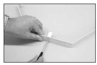
☐ 3) The main landing gear - with the nylon mounting block now firmly in place - can now installed to the fuselage using the four provided 8-32 x 14 mm Allen head bolts, four 4 mm flat washers and the four 4 mm split ring washers. **NOTE:** The main landing
