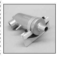
□ 9) The MAC's Products #9114 aluminum exhaust diverter is now fitted to the exhaust tube on the muffler. This diverter uses a
