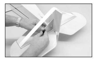
□ 7) With the stabilizer and elevators and the vertical fin permanently in place, unbolt the bottom wing and set it aside. In this step, the elevator control horn is mounted in place to the leading edge of the left inboard elevator. From the kit contents locate one of the three remaining nylon control horns, its nylon base, two M2 x 15 mm Phillips Head bolts and the 3-3/8" elevator pushrod with the clevis in place.
