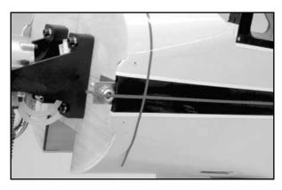
b) Install the cowl back onto the fuselage using the four mounting screws. At the exact rear edge of the cowl in side view, at the black trim stripe, lay another piece of 1/16" trim tape vertically, matching the rear edge of the cowl. Remove the cowl from the fuselage. From the forward edge of the vertical piece of trim tape, measure the distance to the center of the fueling valve and note this measurement on paper (for reference, our
