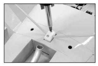
☐ 6) The two main 2-3/4" diameter wheels are now installed onto the wire axle ends. First, slide one of the 4 mm wheel collars
