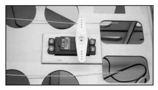
With the servo arm now seated correctly and with the servo moving in the correct direction, the pull-pull cables are now attached to each side of the output arm.
