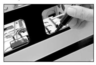
☐ 2) Using scissors, cut out each individual window, leaving about 1/8" of plastic around the edges for a gluing surface. When all four windows are cut out, test fit each of them into their respective openings. Pop them back out and use a little alcohol and a paper towel to clean the gluing edges of each window.
