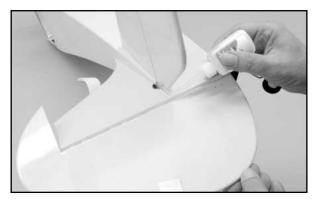
After sufficient time has passed, briskly flex the rudder left and right to free up its movement. Any excess glue can be removed with SIG Debonder.
