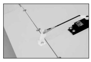
☐ 11) The four top wing N-strut mounting brackets (two per wing panel) are now installed into the bottom surfaces of top wing panels. These brackets are factory-painted yellow and have "closed" angles bent into them, as shown. Just as we did earlier with the bottom wing brackets, these top wing brackets are installed into the recesses built into the bottom surfaces of the top
