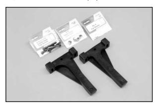
The first step is to properly mount the engine itself to the motor mount arms. An easy and accurate way to do this is to temporarily mount the two motor mount arms onto a scrap piece of 1/8" lite-ply, cut to a 3-1/2" square. Doing this ensures that the back faces of both mounts are truly flat in relationship to each other and the engine when it is eventually mounted in place to the firewall.
