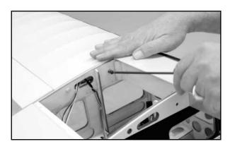
Make the aileron and flap connections with the Y-harness leads in the fuselage. Tuck the excess servo cable back into the wing roots. Use your transmitter to now, once again, test the movement of the ailerons and flaps. Turn off the radio system once you're satisfied.
