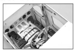
Once all connections have been made, use the transmitter to test each fuselage mounted servo. If you have installed a glow driver system, now is the perfect time to program it. We set ours up to light the glow plug up to 1/4 throttle through our transmitter and we have never felt the need to change this initial program.
