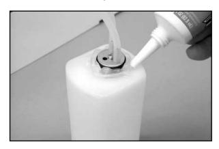
From the bottom wing saddle opening on the fuselage, insert the tank into the tank compartment. Feed the two silicon fuel lines through the round opening in the firewall, and then push the fuel tank firmly in place against the backside of the firewall. Press the tank firmly, compressing the silicon sealer to make a good seal.
