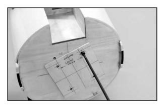
then through the corresponding hole in the firewall. Engage the threads of the blind nut being held in place and begin threading it in place. Keep pulling back on the bolt, holding the blind nut against the firewall, while threading it fully in place. Use an Allen wrench to continue tightening the bolt, pulling the blind nut fully into the backside of the firewall. Remove the bolt and repeat this process to install the remaining blind nuts.
