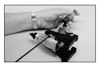
Apply a little threadlock compound to each of the  $8-32 \times 25$  mm mounting bolts. Slip a split ring washer and a flat washer onto each mounting bolt. Hold the engine/motor mount assembly in place to the firewall and install each bolt in place to hold the assembly to the firewall. Allow enough play in the bolts to be able to slide the motor mount arms left or right, as needed, to center the motor mount bases to the firewall. When everything looks about right, firmly tighten the bolts.
