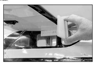
Because of the Waco's two wings and generally large size, the use of a balancing fixture is not very practical. However, you can either balance the model from the wing tips using the 5/16" measurement - taken from the back edge of the bottom main wing spar - or you can balance the airplane at the marks made against the fuselage, using your fingertips. Note that the model is always balanced with the fuel tank empty.
