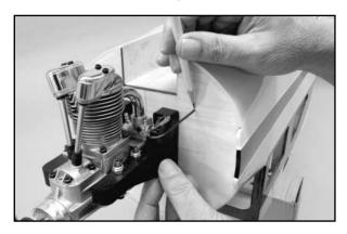
d) The outer nylon throttle housing tube is now installed. First, lightly sand the tube with #220 sandpaper to roughen its surface a bit. Insert the tubing into the firewall, feeding it all the way back toward the throttle servo. Using 5-minute epoxy, glue the tube to the firewall, leaving 3/4" of its length protruding from the face of the firewall. Allow the glue to cure.
