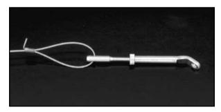
Pull the looped cable and swage through the turnbuckle hole, closing the loop to within about 3/32" - 1/8". Firmly crimp the copper swage, locking the cable in place. Use a small side-cutter to clip the 1/8" of cable - bent at  $90^\circ$  - leaving about 1/16" or so.
