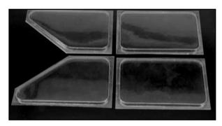
We suggest using 5-minute epoxy glue to mount these windows. **Do not** use CA glue for this purpose! Apply a thin bead of glue around the gluing edges of the plastic window and press it in place from the inside of the fuselage. If necessary, use a few small pieces of tape to hold the window in place until the glue sets. A
