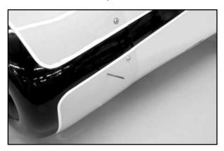
At the outside of the cowl, use a fine tip marker to mark the wire about 1/8" or so away from the cowl itself. Once again, unthread the needle valve and remove it and the wire from the cowl. Use a heavy set of pliers to bend the wire 90° at the mark just made. Use a carbide cut-off wheel to trim the bent end of the wire to a length of about 1/2" or so. You should now have accurately located and usable needle valve extension.
