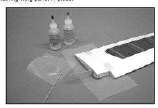
□ 3) After the glue has set, use the four provided 1/4" x 10" self-adhesive strips of white Oracover® film to cover the bottom and top wing joints, centering the covering over each joint. Save the excess strip material. Check the fit of the completed wing to the fuselage. Remove the wing and set it aside for now.
