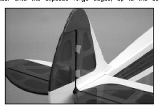
inserts. Remove one of the spacers, flex the rudder over to one side and apply 3 or 4 drops of thin CA glue to the exposed center of the hinge. Turn the fuselage over and apply another 3 or 4 drops of glue to the other side of the hinge. Repeat this operation on the remaining rudder hinge. Allow about 10 minutes before flexing the hinges.
