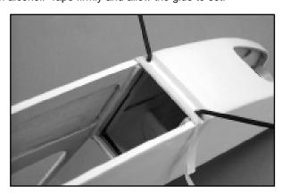
□ 8) Locate the pre-covered battery hatch from the kit contents. This hatch has a plywood "lip" at one end, and two pre-drilled holes at the other end. The end with the lip is the front. The hatch fits into the bottom of the fuselage and is removable for ready access to the battery pack. Install the front lip of the hatch into the fuselage, beneath the landing gear spreader, pressing it firmly up to the back edge of the spreader. Now press the rear of the hatch in place to the fuselage.
