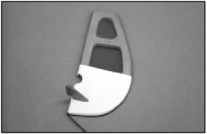
c) The tailskid wheel pant halves are glued to each side of the tailskid wire. Hold the pant halves in place with the tailskid wire between them. Pinch the halves hard to leave the wires' impression on the inside faces of the pant halves. Use a hobby knife to open up the impressions just a little, allowing the wire to "nest" in place between the pant halves. The pant halves are now glued in place, sandwiching the tailskid wire between them. Use SIG thick CA or 5-minute epoxy for this step.
