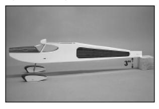
□ 3) Press one of the nylon landing gear clips onto the upright wire leg of the landing gear, immediately next to the wheel pant. Slide the clip up or down on the wire until the boltholes are approximately 3/8" above the axle hole. Use a sharp pencil to
