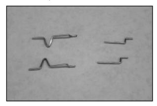
Use a soldering iron and solder to connect the servo linkage ends with each of the two control cables. This is done by using the 1/16" x 1/4" brass tubes, provided in the kit, to couple the wire ends to the cable ends. Use just a small amount of solder to "sweat" these joints.
