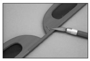
□ 3) The elevators can now be hinged in place to the horizontal stabilizer. The supplied hinges are the CA type. Instant or "thin" CA glue is used to install these hinges.
