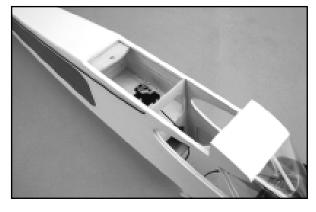
□10) The battery pack is held securely in place during flight with the 3-1/2" length of Velcro® tape provided in the kit. Pull the two Velcro® strips apart, remove the protective backing from the tape side and stick one strip to the bottom of your battery pack and the other strip to the floor of the battery hatch.
