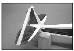
☐ 6) Before hinging the rudder to the vertical fin, it must first be prepared. There are three steps that must be done: a) mount the tailskid wire to the rudder b) glue the rudder control horn in place and c) glue the tailskid wheel pant halves to the tailskid. Locate the rudder, the rudder control horn, the tailskid wire, and the two wheel pant halves.
