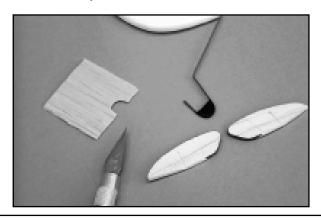
□ 7) The rudder is now ready for hinging to the vertical fin with two CA hinges. The procedure is exactly the same as those for hinging elevators back in Step 3. Insert the two hinges into the vertical fin, with their center slots aligned with the trailing edge of the fin. Insert thin scrap wood or cardboard into these slots to keep them centered and from being pushed further into the fin. Slide the rudder onto the exposed hinge edges, up to the scrap
