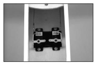
Run the cables through the tubes until they exit the fuselage at the rear. Position the servo arms squarely to the servos and reinstall them back onto the servos.
