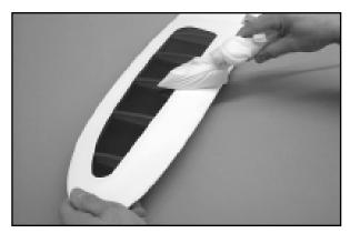
A very easy way to avoid damaging seams and joints when reshrinking the covering is to protect the seams with wet paper towels rolled into strips. These are arranged directly onto the joints or seams and their coolness protects the seam from shifting or "crawling" under heat.
