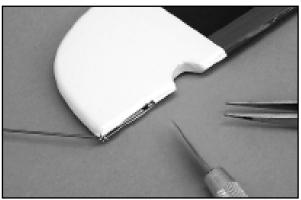
b) Like the elevator control horn, the rudder horn is glued into the pre-cut slot at its bottom leading edge on its' left side, as shown. First, find the slot location beneath the covering - approximately 5/8" above the bottom edge of the rudder. Use a hobby knife to cut through the covering, exposing the slot. Use 5-minute epoxy to glue the horn into the slot and allow the glue to cure.
