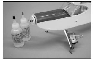
Use light sandpaper (#400 or so) to lightly sand the trailing edges smooth and sharp. The fairings can now be finished in either paint or covered with Oracover® film. Remount the wheel pants.
