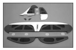
□ 2) Before hinging the elevators to the horizontal stabilizer, glue the elevator control horn in place first. Make sure the three (3) drilled holes are cleared out. Use a pin or small diameter drill to do this.
