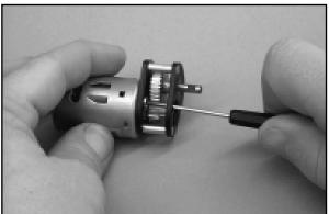
□ 2) The SIG Electronic Speed Controller (ESC) has been factory soldered to the motor for your convenience. **NOTE:** The gearbox reverses the direction of rotation of the propeller shaft. Therefore the white wire (normally negative) has been soldered to the positive tab on the motor and the red wire has been soldered to the negative motor tab. This provides the correct direction of rotation for the propeller.
