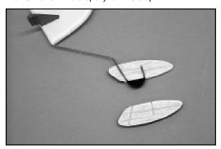
**MODELER'S TIP:** The overall look of the tailskid/wheel pant assembly can be easily enhanced by filling in the exposed "wheel" part of the wire with a small scrap piece of 1/32" balsa. Use thin CA to glue the wood in place, sand the sides smooth to the wire and paint with flat black paint. The finished product will look just like a tail wheel!
