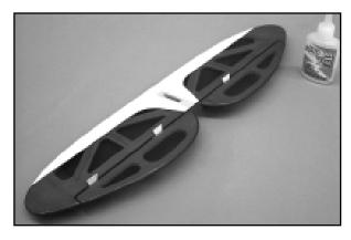
□ 4) With the elevators in place, the horizontal stabilizer is now glued in place to the top rear of the fuselage. Use SIG 5-minute epoxy for this operation.
