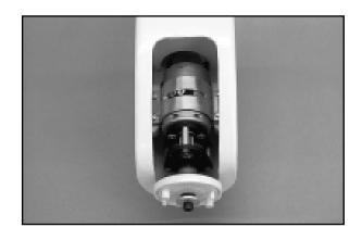
The motor/gearbox is now locked in place by tightening the four motor mount screws. Position the spinner backplate with approximately 1/16" - 3/32" clearance between its rear face and the front of the fuselage and be sure the propeller shaft is centered. Now tighten the motor mount screws. We strongly suggest that you do not mount the propeller in place until you are ready to go flying.
