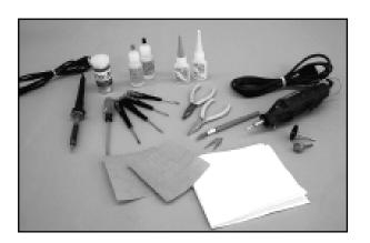
You will also be required to make a few solder connections. We suggest that you have a good soldering iron and good quality solder and flux. For the pushrod connections, we use and like the Stay-Brite® Silver Solder products. For electrical connections, use solder specifically for that purpose.
