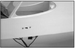
mounting plate to the inside of the fuselage, aligning its slot with the slot in the fuselage. The plywood plate provides a hardpoint for the switch. Using the screws provided, mount the switch in place into the fuselage. Do not over-tighten the switch mounting screws.
