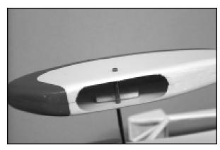
□ 2) The wheel pants must first be correctly aligned to the landing gear wire and the fuselage, before mounting. This is done by slipping the wheel pants in place over the landing gear wires - without installing the wheels - and then propping the rear of the fuselage up 3" off of a flat surface. This provides the correct side view alignment for mounting the wheel pants.
