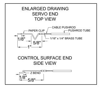
☐ 5) Use a small screwdriver to remove the servo control arms from the servos. Install the wire linkage "Z-bend" ends of the control cables onto the servo control arms. Install the two control cables into the two plastic tube ends in the servo compartment.
