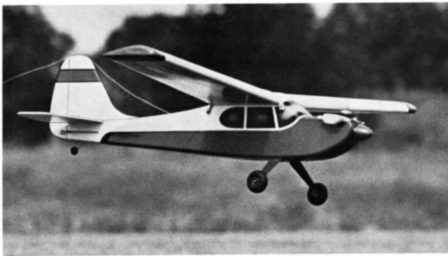
Prototype Scamp #1 on a landing approach. The wing on this model is painted with SIG PLASTINAMEL, and the fuselage and tail surfaces are painted with SIG SUPERCOAT DOPE. Power is an O.S. Max .15.
